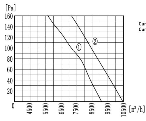
Curve 1: 50HZ Curve 2: 60HZ
